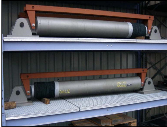
Fig. 30: MHD´s ready for installation with assembly brackets
