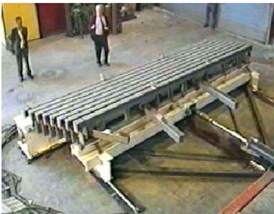
Fig. 52: Tests of a seismic swivel-joint expansion joint of Type DS at the Berkeley University - CA
