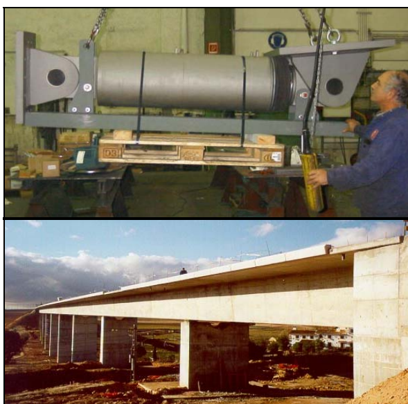
Fig. 26: 2.500 kN MSTL for railway viaduct De La Rambla in Spain
