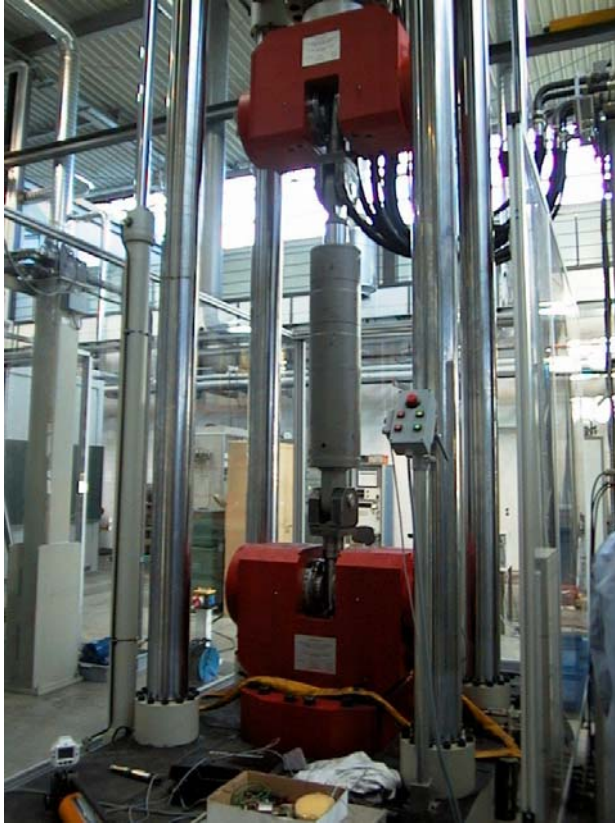
Fig. 50: Tests of damper (MHD) and shock transmitter (MSTU) at the Technical University Munich
